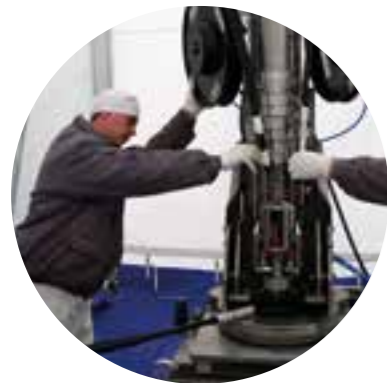
Kozloduy NPP Design and manufacturing of equipment to take ion exchange resin samples
