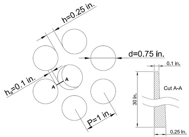
**Figure 1. Mis-Drilled Hole Geometry**
