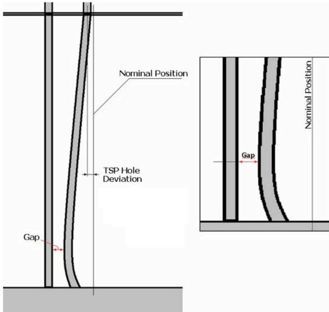
**Figure 3. Tube-to-Tube Clearance**
