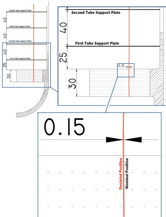
**Figure 2. Tube Configuration with TSPs and Tubesheet**
